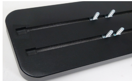
(Fig 16) Slip M6X1-20mm Square Head Bolts Into The Bottom Channels
